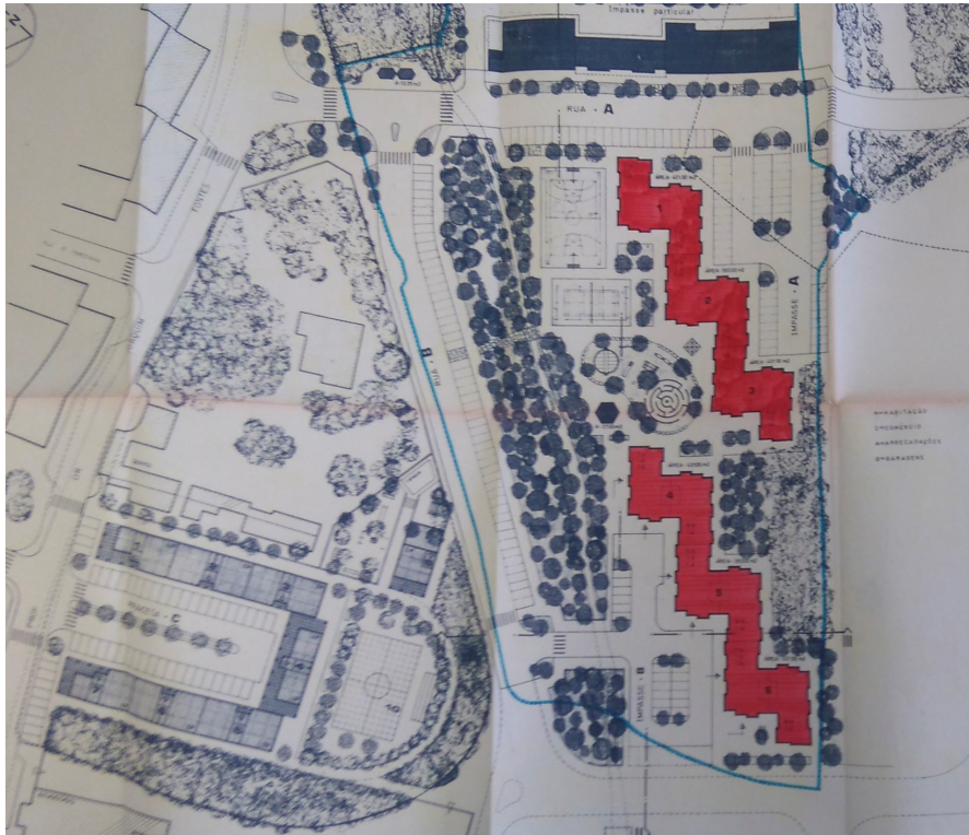
Fig. 30 – Multifamily buildings with commercial and services use typology allotment permit in Mem Martins (10 plots, 162 homes)
